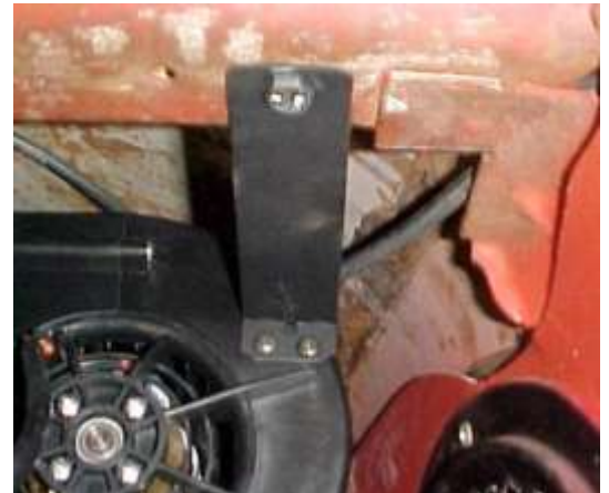
STUD BRACKET FROM INSIDE OF THE CAR
