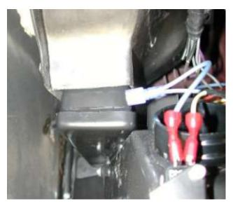
Insert (1) upper rear Evaporator mounting stud through the original hole as shown. Attach using (1)  $\frac{1}{4}$ " – 20 flange nut provided.
