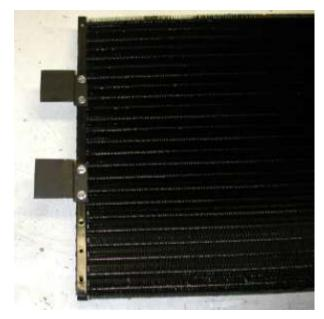
Locate the Condenser, (2) right condenser mounting brackets, and (4)  $\#10 \ge 3/8$ " hex head screws.
