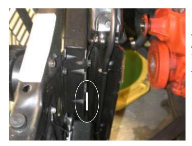
The (4) condenser mounting brackets are clamped between the radiator and its mating bulkhead.
