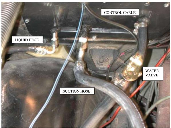
Locate the water valve and (3) worm gear clamps from the hardware sack kit. Cut 6" of heater hose from the **RETURN HOSE**. Attach this piece to top fitting
