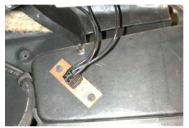
Locate behind original control head the resistor connector, on heater box.
