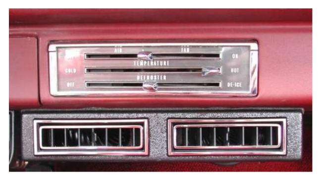
THE PICTURE YOU SEE ABOVE SHOWS THE CONTROLS IN THE DEFROST MODE. THIS MEANS THAT THE AIR WILL BE DISTRIBUTED THROUGH THE DEFROST OUTLETS. THIS ALSO HAS THE TEMPERATURE LEVER IN THE HOT POSITION. WITH THE CONTROLS IN THIS POSITION YOU WILL GET THE AIR THROUGH THE DEFROST OUTLETS WITH THE COMPRESSOR ON.
