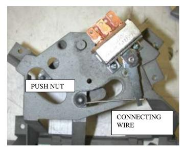
Locate the blower switch, (2)  $\#6 \ge 3/8$ " pan head screws, (1) 3/16" push nut and connecting wire from the control sack kit.
