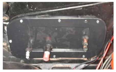
Locate the Firewall Block Off plate, and (6)  $\#10 \times \frac{3}{4}$ " hex head tek screws.
