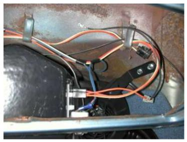
Attach (2) blue wires to the micro-switch and blue pig tail located next to the face / heat door crank arm. Refer to wiring diagram for correct connections.
