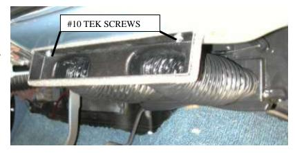
Attach 7 <sup>1</sup>/<sub>2</sub>" flex hose between center hose adapter and the distribution duct adaptors.
