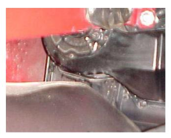
Remove (7) screws around the perimeter of the Blower Housing. The (2) screws around blower motor can be accessed from below and between the fender well and fender. Remove blower assembly.
