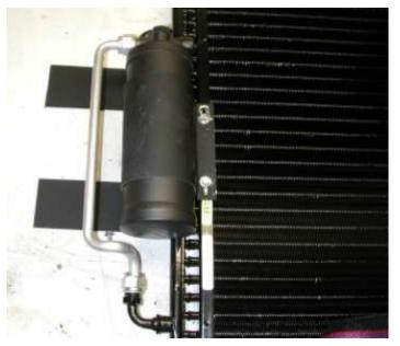
Locate Filter / Drier, Drier Mounting Bracket, Aluminum Liquid tube, (2) #6 orings, and (2) #10 x 3/8" hex head screws.
