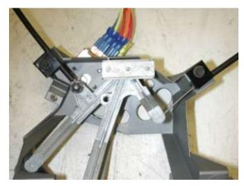
Attach (longest) temperature control cable using original hardware to the CENTER control arm and (1) 3/16" push nut. NOTE: Cable sleeve is 1/16" from the lever arm.
