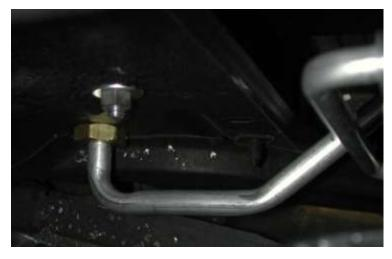
Rotate lower fitting up to the radiator bulkhead. Locate and drill (1) hole 13/16" diameter.
