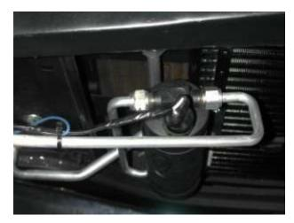
Locate liquid tube, Hi / Low pressure switch assembly, wire harness, (1) #6 o-ring, tube support bracket, # 6 tube clamp, (1) #8 x 3/8" screw and (1) #8-32 x 3/8 screw and nut.
