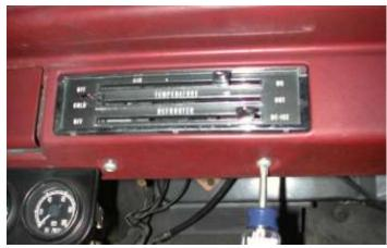
Remove control head and disconnect the electrical connector. Also disconnect (3) original control cables retain the original hardware.
