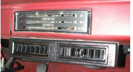
Locate Center Louver Bezel Assembly and (2) #8 x 3/8" pan head screws.
