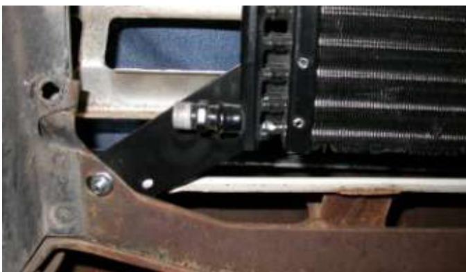
VIEW SHOWING UPPER BRACKETS FROM GRILLE SIDE OF BULKHEAD.
