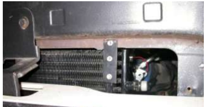
VIEW SHOWING UPPER BRACKETS FROM GRILLE SIDE OF BULKHEAD.
