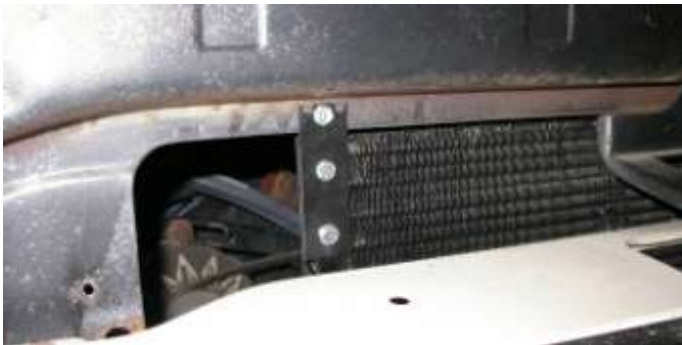
VIEW SHOWING UPPER BRACKETS FROM GRILLE SIDE OF BULKHEAD.
