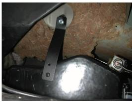
Insert hookup tubes through the original heater motor hole.
