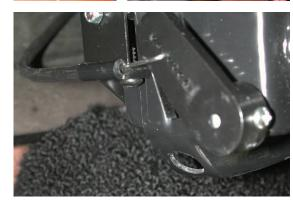
Locate (1)  $\#10 \times \%$ " tek screw and (2)  $\#8 \times 3/8$ " pan head screw from the hardware sack kit.
