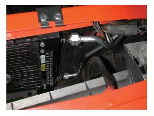
Locate the (2) upper condenser mounting brackets, (4) #10 x 3/8" hex head screws, (4)  $\frac{1}{4}$ "-20 j-clips and (4)  $\frac{1}{4}$ "-20 x  $\frac{5}{8}$ " hex head screws.
