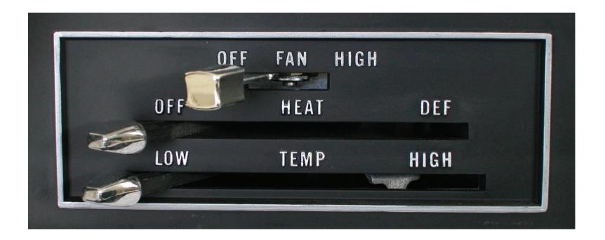
THE PICTURE YOU SEE SHOWS THE CONTROLS IN THE HEAT MODE. THIS MEANS THAT THE AIR WILL BE DISTRIBUTED THROUGH THE HEATER OUTLETS. THIS ALSO HAS THE TEMPERATURE LEVER IN THE COLDEST POSITION. WITH THE CONTROLS IN THIS POSITION YOU WILL GET THE AIR THROUGH THE HEATER OUTLETS AND THE OUTLET TEMPERATURE AT THE COLDEST POSSIBLE DEGREE.
