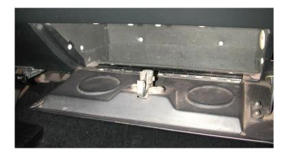
Locate the under dash louver assembly and (2) pieces of 2  $\frac{1}{2}$ " dia. flex hose 9" long, (1) piece of 2" flex hose 48" long, (2) snap in hose adaptor and (3) #10 x  $\frac{3}{4}$ " tek screws.
