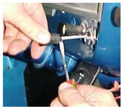
Remove the control knob as shown.
