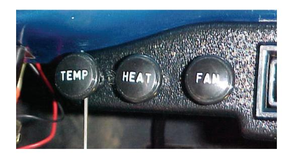
THE PICTURE YOU SEE SHOWS THE CONTROLS IN THE HEAT MODE. THIS MEANS THAT THE AIR WILL BE DISTRIBUTED THROUGH THE HEATER OUTLETS. THIS ALSO HAS THE TEMPERATURE LEVER IN THE COLDEST POSITION. WITH THE CONTROLS IN THIS POSITION YOU WILL GET THE AIR THROUGH THE HEATER OUTLETS AND THE OUTLET TEMPERATURE AT THE COLDEST POSSIBLE DEGREE.
