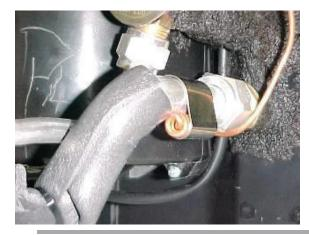
Locate in the hardware sack kit the small #6 liquid tube.
