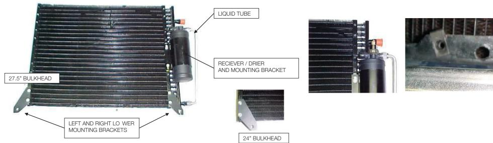
NOTE: VEHICLES EQUIPT WITH 27.5" RADIATOR BULKHEAD ATTACH LOWER LEFT BRACKET AS SHOWN IN THE LEFT PICTURE. THOSE EQUIPT WITH 24" RADIATOR BULKHEAD ATTACH AS SHOWN IN THE RIGHT PICTURE.
