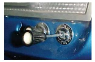
Located on top of the heater assembly remove defrost ducts and discard. Also disconnect control cable and discard the hardware.
