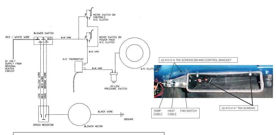
WIRING DIAGRAM 1965 -66 FORD TRUCK
