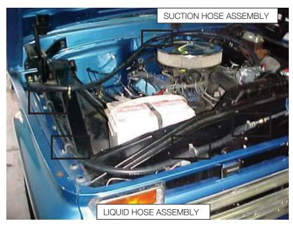
Locate (4) #6 hose clamps, and (4)#10 x 3/4" tek screws.
