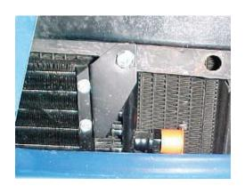
Locate and remove the Hood Latch Assembly. Retain original hardware.
