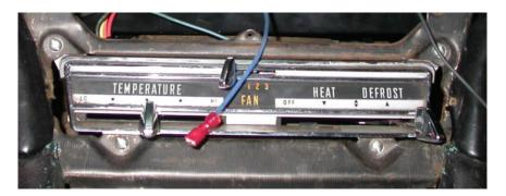
Carefully snap off chrome frame around the control head.
