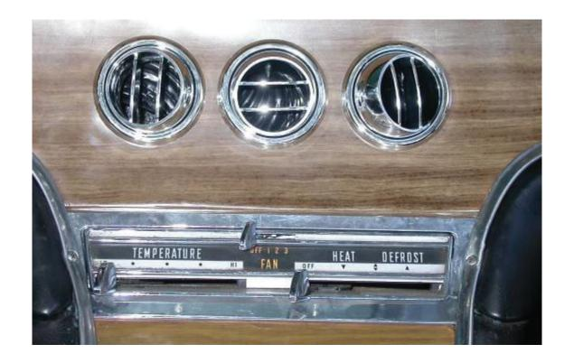
THE PICTURE YOU SEE SHOWS THE CONTROLS IN THE HEAT MODE. THIS MEANS THAT THE AIR WILL BE DISTRIBUTED THROUGH THE HEATER OUTLETS. THIS ALSO HAS THE TEMPERATURE LEVER IN THE COLDEST POSITION. WITH THE CONTROLS IN THIS POSITION YOU WILL GET THE AIR THROUGH THE HEATER OUTLETS AND THE OUTLET TEMPERATURE AT THE COLDEST POSSIBLE DEGREE.
