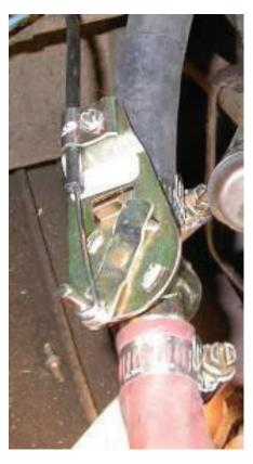
Locate (2) white wires tywraped to the discharge tube. Route along the discharge hose. Cut one of the wires and attach female bullet connector provided and plug into the compressor clutch wire.
