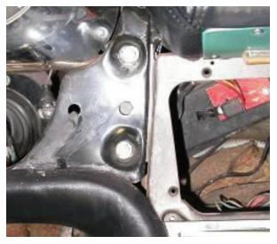
Remove (4) mounting bolts that hold the panel to the dash.
