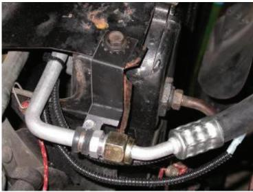
Locate #6 liquid hose and (2) #6 o-rings. Attach hose between fitting on firewall and fitting on the condenser.
