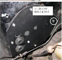
Remove blower motor access cover and remove (4) nuts that attach the heater box to the firewall. Next picture shows location of the nuts. Retain original screws discard the nuts.
