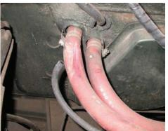
Defrost attachment to diffusers typical drivers and passenger side.
