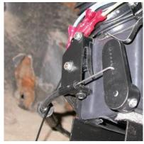
Locate orange wire with bullet connector that was attached to the original blower motor. Cut off the connector and add a ¼" male spade connector.
