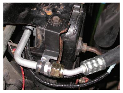
When routing suction hose tywrap hose to the body brace beside the air cleaner.
