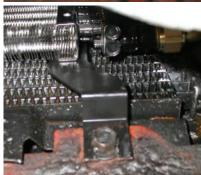
Attach discharge tube to #8 fitting on the condenser using an o-ring and a few drops of mineral oil.
