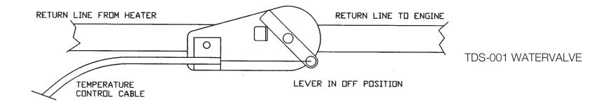
CAUTION: WATER VALVE MUST BE INSTALLED ON HEATER LINE ROUTED TO WATER PUMP.
