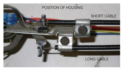
Locate blower switch assembly provided in the kit.
