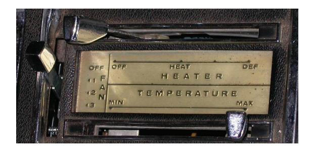
THE PICTURE YOU SEE SHOWS THE CONTROLS IN THE HEAT MODE. THIS MEANS THAT THE AIR WILL BE DISTRIBUTED THROUGH THE HEATER OUTLETS. THIS ALSO HAS THE TEMPERATURE LEVER IN THE COLDEST POSITION. WITH THE CONTROLS IN THIS POSITION YOU WILL GET THE AIR THROUGH THE HEATER OUTLETS AND THE OUTLET TEMPERATURE AT THE COLDEST POSSIBLE DEGREE.
