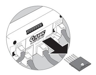
REMOVE CALIBRATION KEY FROM ECU AND STORE IN A SAFE PLACE
