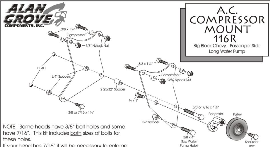
If your head has 7/16" it will be necessary to enlarge the corresponding holes in the mount to 7/16".
