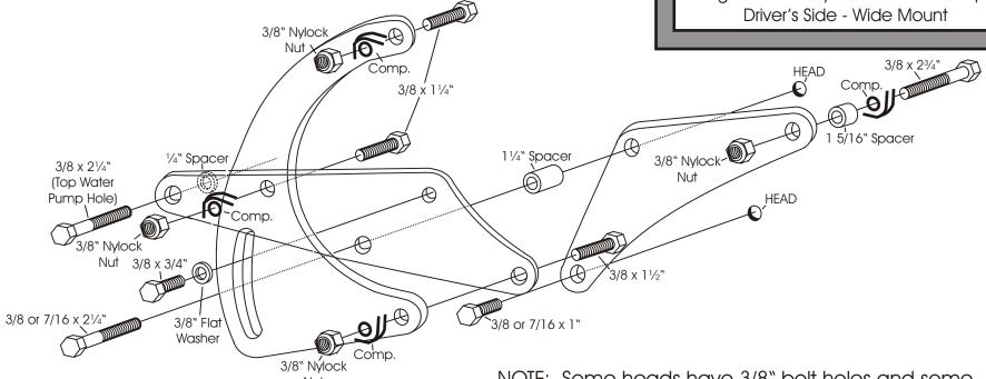
(We use a belt length of 58-59" with this mount on installations in our shop. However; this can vary with the diameter of your pulleys.)
