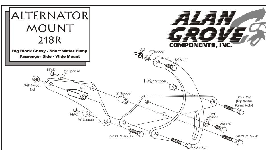
(We use a belt length of 58-59" with this mount on installations in our shop. However; this can vary with the diameter of your pulleys.)
