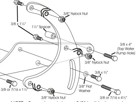
NOTE: Some heads have 3/8" bolt holes and some have 7/16". This kit includes both sizes of bolts for these holes.
