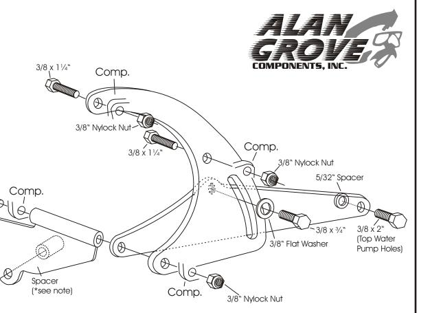
We use a belt length of 60-61" with this mount on installations in our shop. However; this can vary with the diameter of your pulleys.
