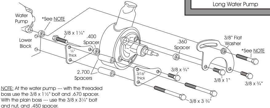
If your pump has a stud at the lower rear pivot point, remove it and use the  $1\frac{1}{4}$ " bolt and .400 spacer.
