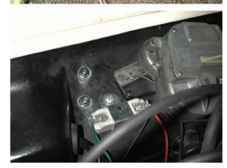
Locate on firewall original hole that the heater valve went through. Enlarge the hole using a 1" drill bit.
