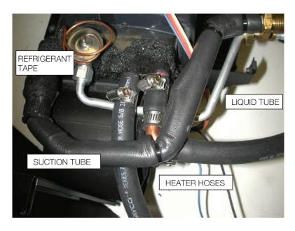
Locate in the hardware sack kit the Suction Tube, Liquid Tube, (1) piece of Heater hose 12" long, (1) piece 18", (2) worm gear clamps, (1) #6, and (1) #10 o-ring.
