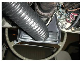
CAUTION: CHECK FOR INTERFERENCE WITH THE WINDSHIELD WIPER CABLES.
