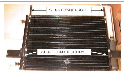
Locate following components from the condenser kit. Condenser, (2) bottom condenser mounting brackets, (2) top mounting brackets, and (8) #10 x 3/8" hex head screws.
