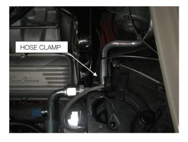
Route discharge hose along fender well and attach end with service port to rear of the compressor, using (1) #8 o-ring and a few drops of mineral oil.
