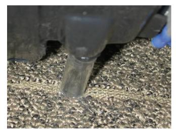
Locate flex hose from the unit and attach to rear of the louver assembly.
