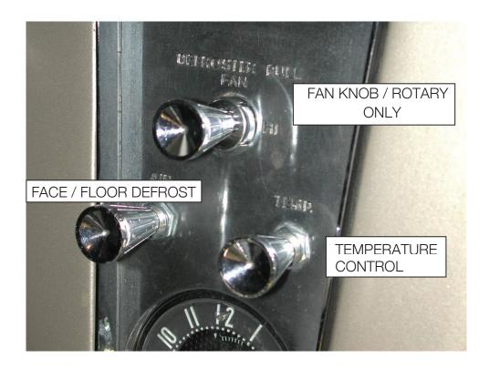
THE PICTURE YOU SEE SHOWS THE CONTROLS IN THE HEAT MODE. THIS MEANS THAT THE AIR WILL BE DISTRIBUTED THROUGH THE HEATER OUTLETS. THIS ALSO HAS THE TEMPERATURE LEVER IN THE COLDEST POSITION. WITH THE CONTROLS IN THIS POSITION YOU WILL GET THE AIR THROUGH THE HEATER OUTLETS AND THE OUTLET TEMPERATURE AT THE COLDEST POSSIBLE DEGREE.
