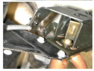
Locate on the end of blower assembly the defrost / heat duct. Remove and discard the original hardware.
