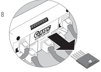
REMOVE CALIBRATION KEY FROM ECU AND STORE IN A SAFE PLACE
