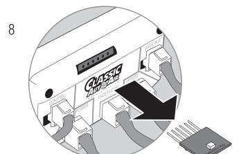
REMOVE CALIBRATION KEY FROM ECU AND STORE IN A SAFE PLACE
