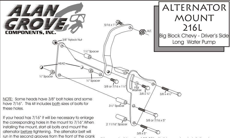
(We use a belt length of 52-53" with this mount on installations in our shop. This was determined using GM Part #14025185 Crank Pulley and GM Part #14023155 Water Pump Pulley.)
