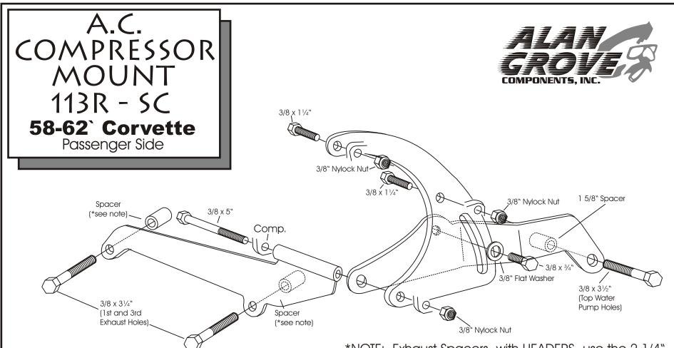
We use a belt length of 60-61" with this mount on installations in our shop. However; this can vary with the diameter of your pulleys.
