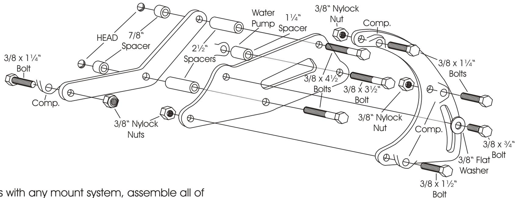
As with any mount system, assemble all of the brackets to engine BEFORE TIGHTENING THE BOLTS.
