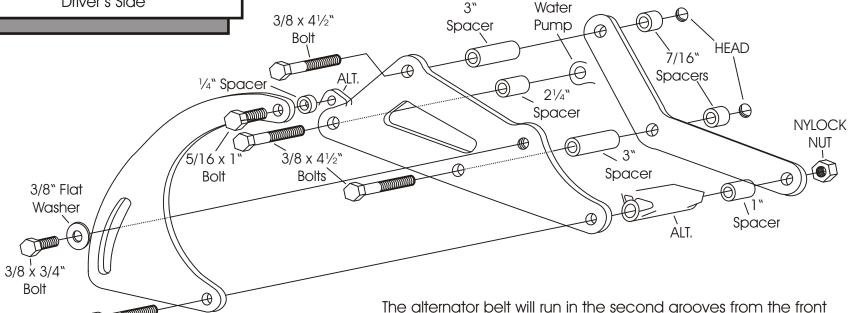
It can be used with single groove crank and water pump pulleys by using a double groove alternator pulley and running the belt in the outer groove.
