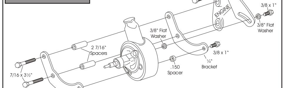
This bracket is designed to be used with the non-metric Chevrolet pump with attached reservoir. There are a large number of pumps available from 1961 to 1981 that will work well with our power steering bracket. For more detailed information see the enclosed power steering pump sheet. Most short water pump applications use a crankshaft p.s. pulley that bolts over the existing pulley. This will align with the p.s. pump pulley. This pulley is available from G.M. as part number- 3751232 or from us.
