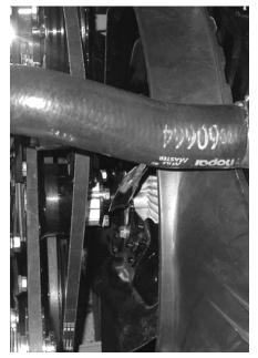
Reinstall the original fan, fan shroud, and water pump pulley.
