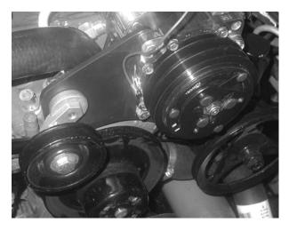
Install the 1 7/8" idler eccentric and pulley to the front vertical. Using (1)  $\frac{1}{2}$ "-20 x 1" bolt.
