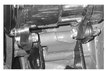
Attach the compressor to the front vertical using (3) 3/8"- $16 \times 1\frac{1}{2}$  bolts and ny-lock nuts.
