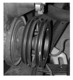
Remove fan, fan shroud, and water pump pulley.
