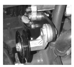
Install the idler eccentric and pulley to the front vertical. Using (1)  $\frac{1}{2}$ "-20 x 1" bolt.
