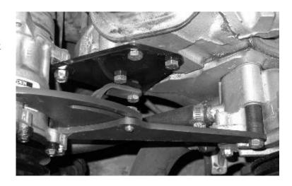
Attach compressor to the front bracket and the adjusting bracket, and rear support brace. Use the 3/8" x 2" bolt and nylock nut as shown.
