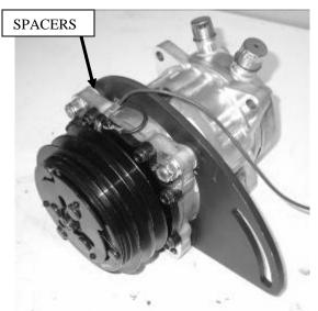
Loosely attach the ADJUSTING bracket to the compressor using (2) 3/8 -16 x 1 ½" bolts, (2) ¼" spacer, and (2) ny-lock nuts as shown.
