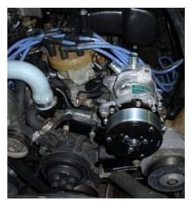
8. Install the 3/16" spacers between the adapter brackets and the mounting ears of the compressor. This will ensure correct belt alignment. Tighten all bolts.
