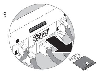
REMOVE CALIBRATION KEY FROM ECU AND STORE IN A SAFE PLACE
