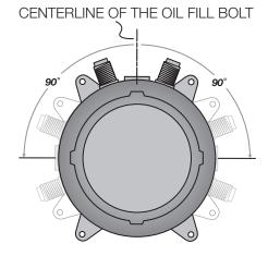
When mounting your compressor and/or adjusting the belt, Set compressor at 90 degrees.
