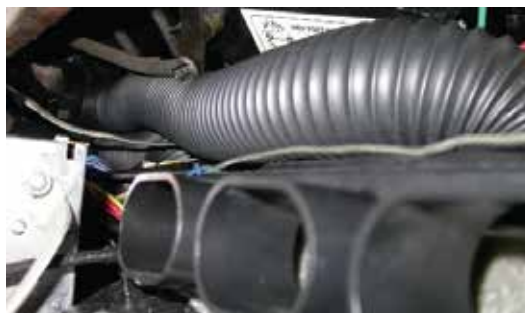
35" HOSE WITH DEFROST ADAPTOR DRIVERS DEFROST DIFFUSER
