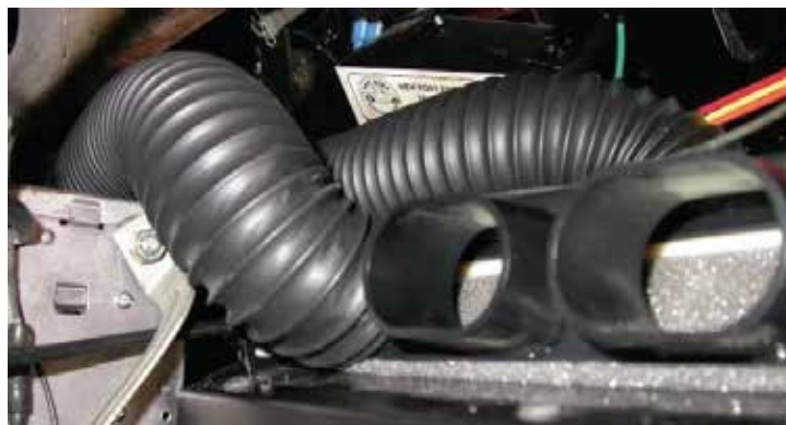
ROUTE 43" HOSE OVER RADIO AND OVER TO THE DRIVERS LOUVER
