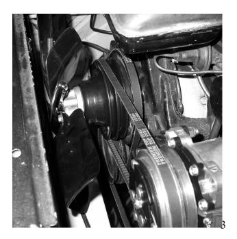
Install the compressor drive belt on the front groove of the compressor and water pump pulley. Tighten all belts to the proper tension.
